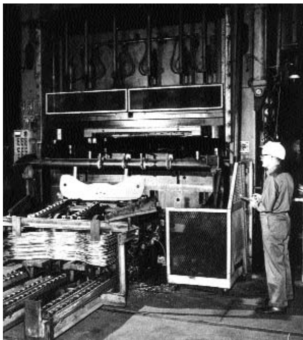
Figure 1- Pumping effect sank foundation of 800-ton press
