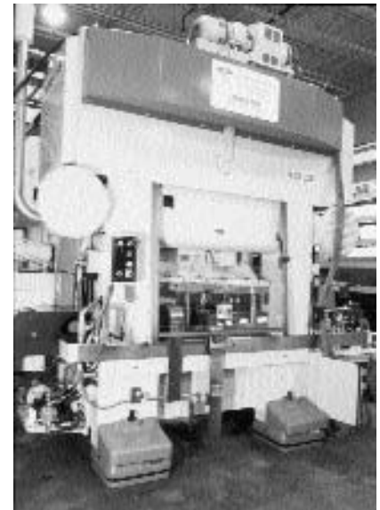
Installation of a high-speed press on VSML Isolators
