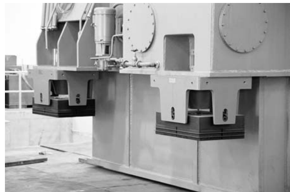
Isolators secured to press bed.
